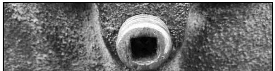
This is the original bell housing drain pipe plug. It is diagnostic plug and does not drain the transmission reservoir.
