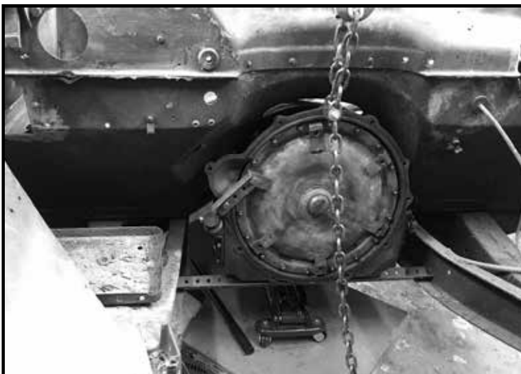
Using hydraulic tools, the transmission is moved until it sets on the rear mount so fastening bolts can be installed. Small piece of angle iron holds torque converter and we create a temporary front mount with angle iron resting on chassis rails.
